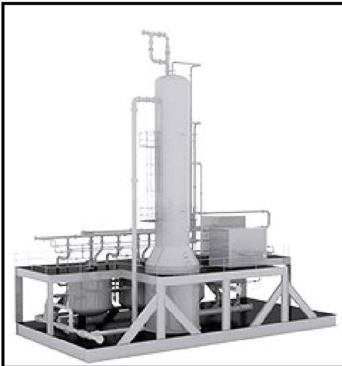
NOV Mission Production Technologies seawater treatment compact system for injection to maintain reservoir pressure. The package includes media filtration and vacuum strip deoxygenation tower.
