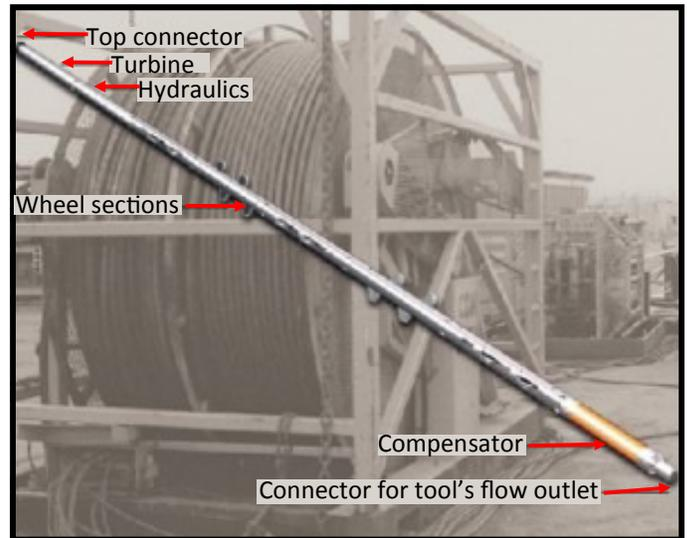
Coiled Tubing Tractor for pulling logging, completion and work over tools.
